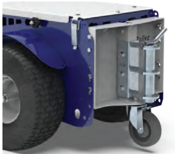
Drop pin hitch Ø16 / 20 / 35 / 40 mm
